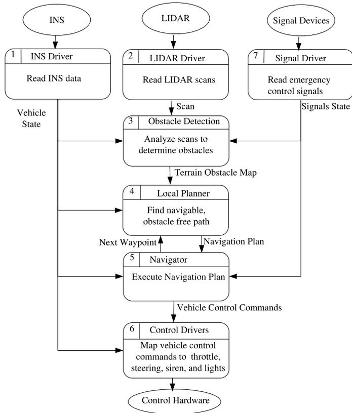
Figure 8: System Level Data Flow Diagram
