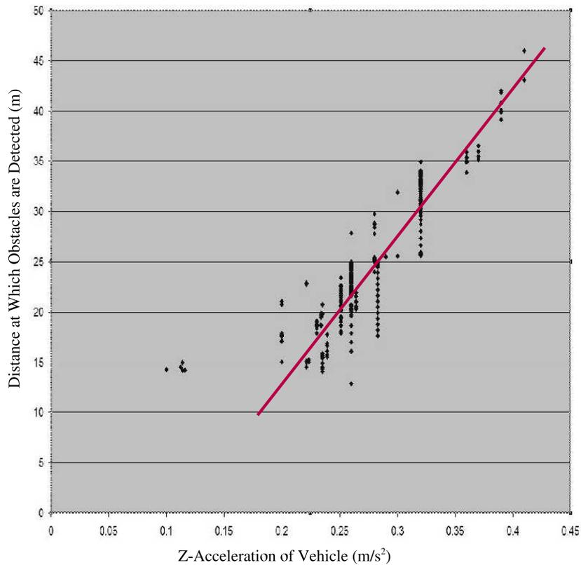
Figure 11: Graph Showing Distance to Detected Obstacles Versus Z-Acceleration
