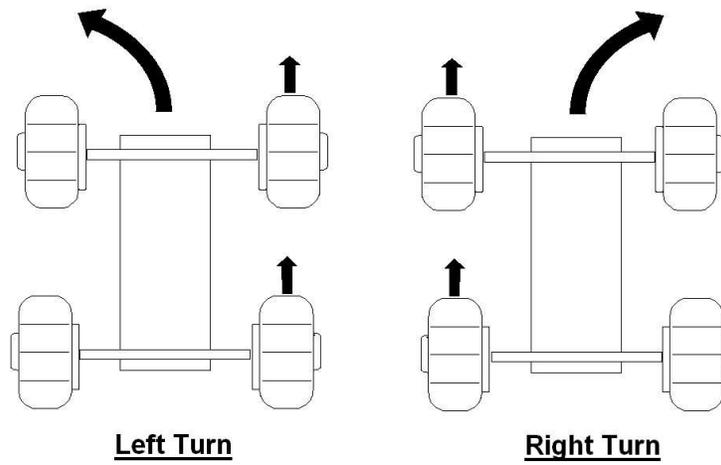
Figure 2: Skid Steered Vehicle
