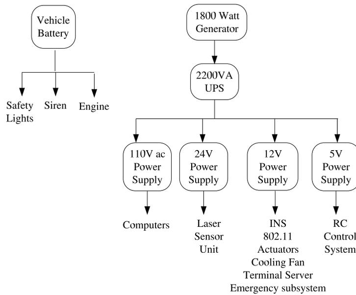
Figure 3: CajunBot E-Power Subsystem
