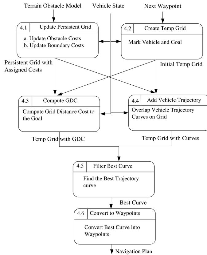
Figure 13: Data Flow Diagram for the Navigator Module
