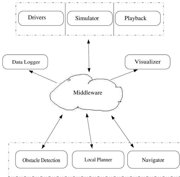
Figure 6: Software Architecture
